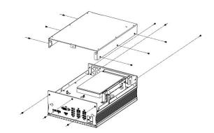
For slots inside the AMI221 & AMI222, you also need to disassemble the intermediate plate by removing the front I/O cover first and then removing 8 screws as shown below.
