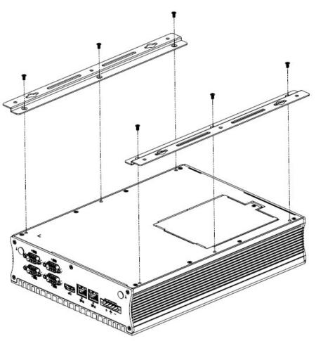
2. Prepare at least 4 screws (M3) to mount the system to the desired wall or location.
